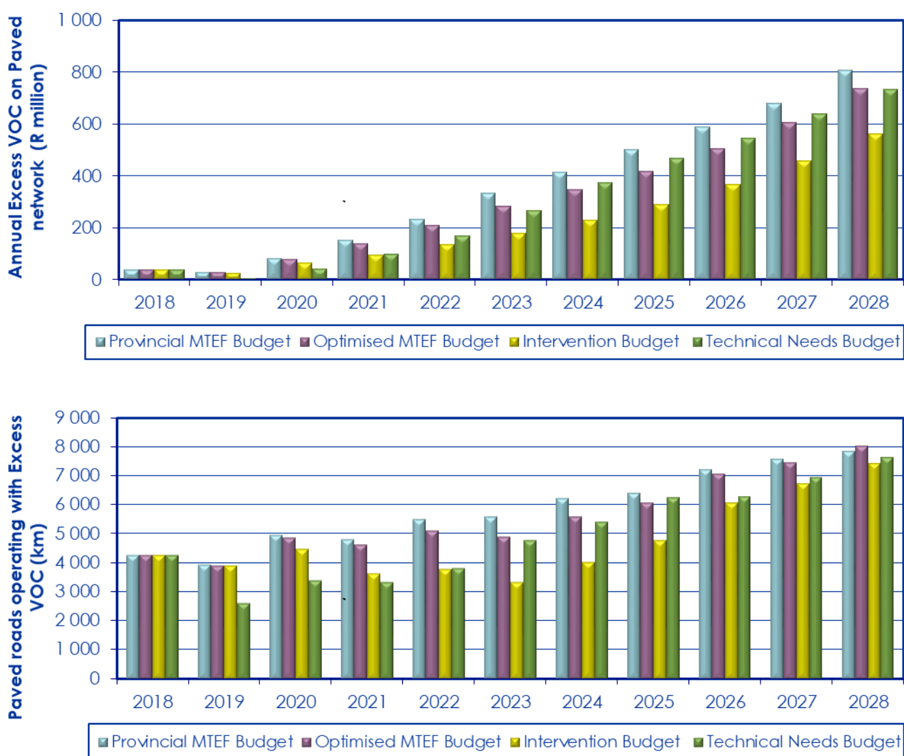
Figure 5-34: Total excess vehicle operating costs in terms of (a) annual cost and (b) km
